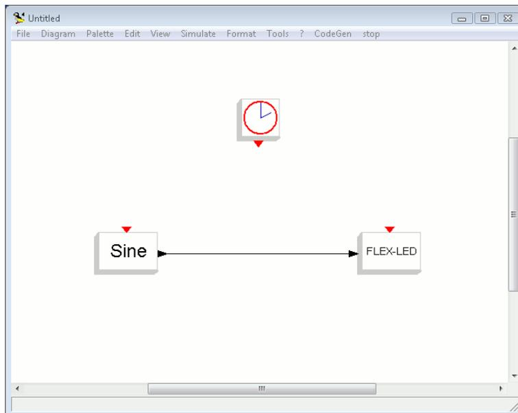
Figure 5.9: Put the clock block over the Sine and LED blocks.
