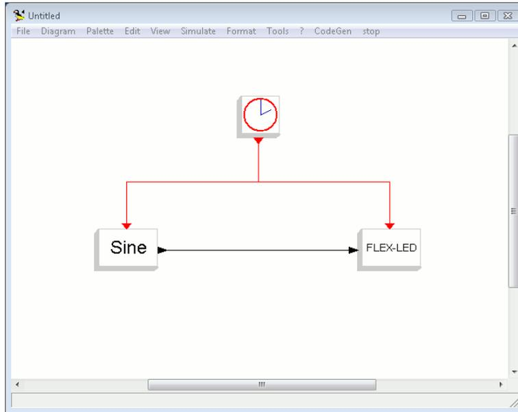
Figure 5.10: The `clock` block is connected to the `Sine` and `LED` blocks.
